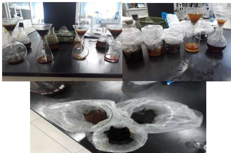
Figure 1 - Filtration process of extracted vegetable extracts
