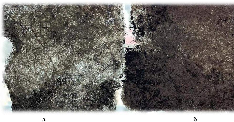
a) sample of untreated material; b) sample of the material treated with brass nanoparticles
